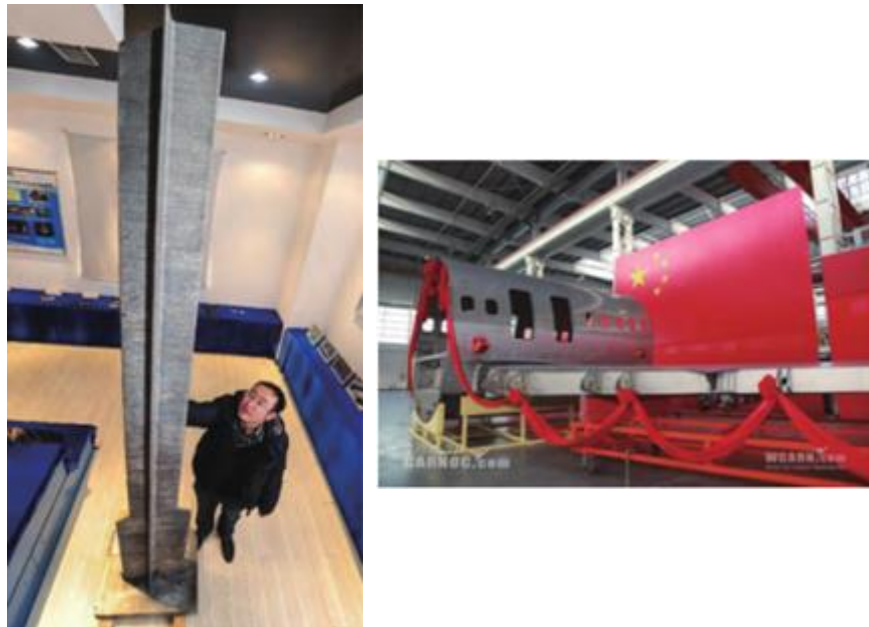
Fig. 1 The upper and lower margins of central wing of the the C919 large passenger aircraft manufactured by Northwestern Polytechnical University
