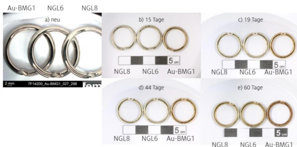
Figure 1: Results of a 60d wearing test of three rings [4]
